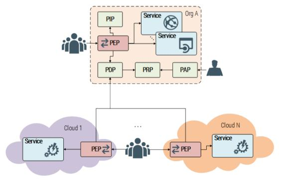
Figure 4: Centralized authorization management in multi-cloud environment
